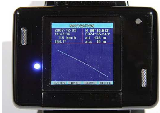
Navigation demo with proper satellite fix shows date, time, speed, true course, position, altitude and accuracy. Also a plot of the path traveled is displayed.
